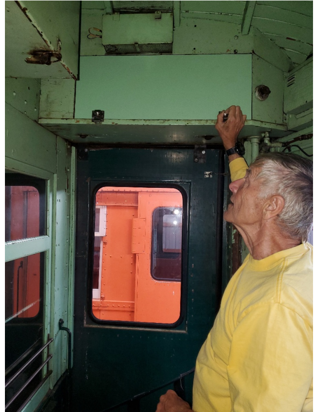
Don Quant is shown here inspecting one of his door engine compartment covers on car 168.
