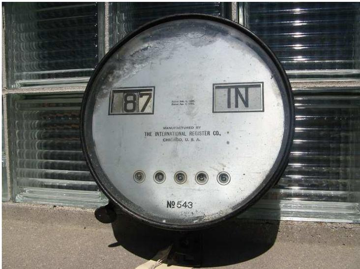
*Fare registers like this International Register Co. model were prominently mounted for conductor (and passengers) to see.*
