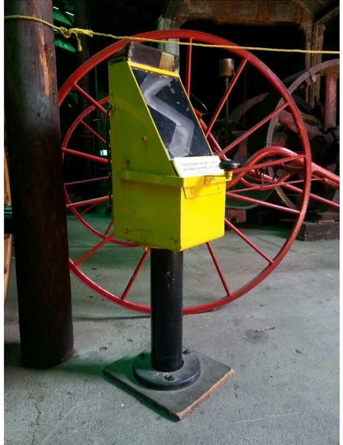
the type, the box is designed to let the bus driver or trolley motorman view the coins as they drop down a zigzag path visible in the photo. At the bottom of this path, the coins rest in clear view until the lever is pushed, dropping the coins into the locked container. Kids enjoy it, and adults are happy to see their change go to a good cause. About the only problem we've had is the occasional ten dollar bill stuffed into the coin opening!
