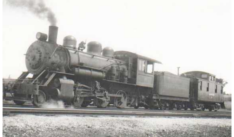
Genesee & Wyoming caboose 8 is seen in this 1938 shot riding on its original DL&W passenger-style trucks.
