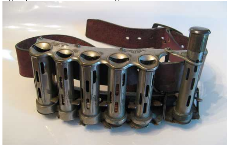
The coin changer has slots for all coins as well as for tokens, and came complete with a belt and over $8 in change!
